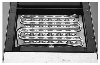
Pour Scale Remover Over The Evaporator Section
